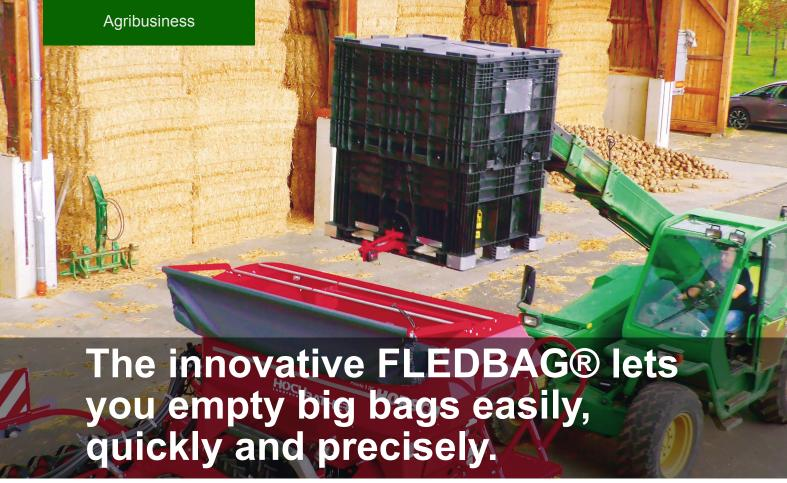
The innovative FLEDBAG® lets you empty big bags easily, quickly and precisely. It is suitable for animal feed, fertilizer, seeds, pellets, salt and granules. Any residual amounts can be left in the big bag for the next dispensing task. FLEDBAG® is available individually or as part of a practical combined package. For reusable big bags we recommend the use of the FLEDBAG® Easy. It was specially developed for use with reusable big bags.
